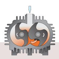
Mink dry claw vacuum pumps and compressors have been developed for use in industrial applications where constant vacuum, high suction capacity and totally oil-free compression are essential. Mink dry claw vacuum pumps and compressors are non-contacting: neither oil or any other operating fluids are required during the compression process.
