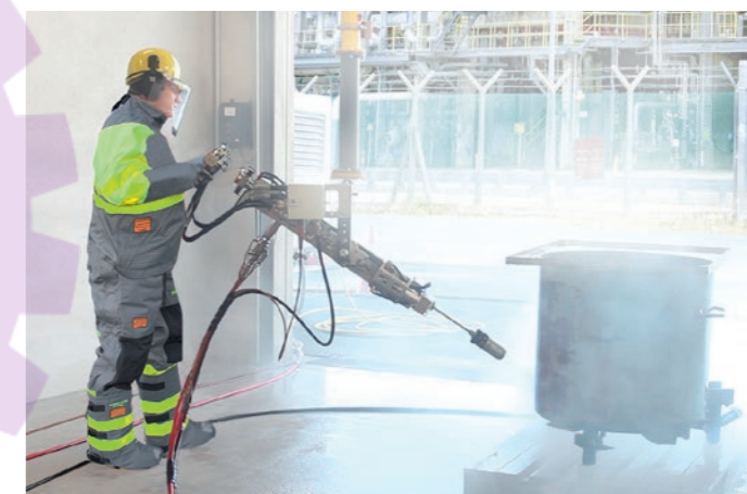
Jetmate - reaction force free jetting tool
