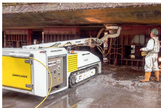
Dockboy - surface preparation on ship hull bottoms
