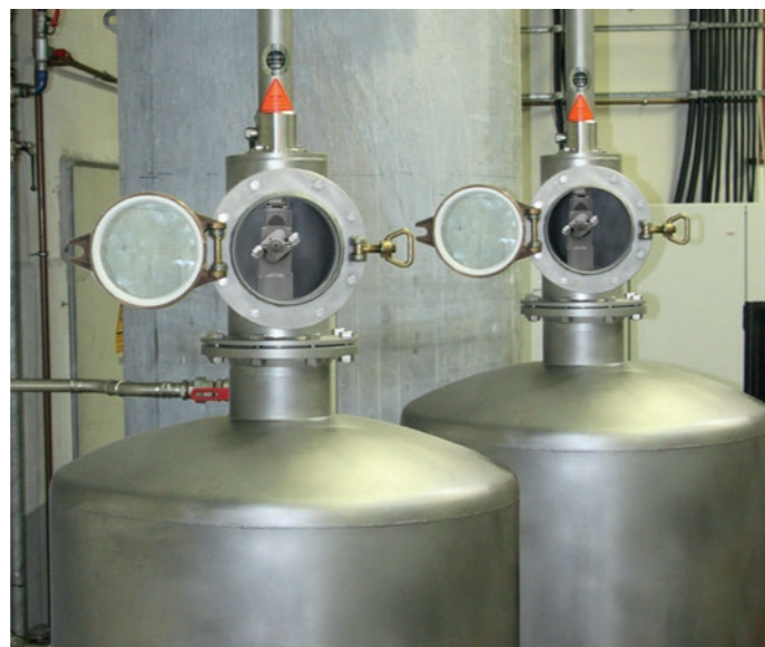
Aquarex - Tank cleaning devices
