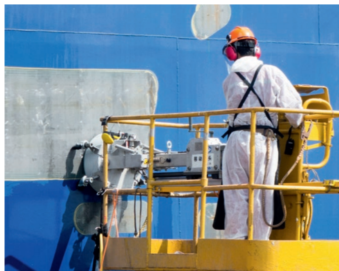
Aquablast Spot - to clean specific small areas
