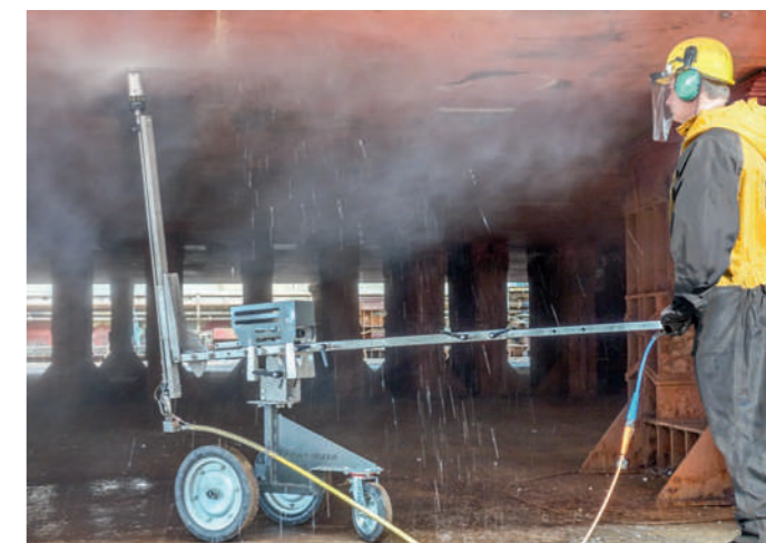
Jetboy - mechanical support for manual work
