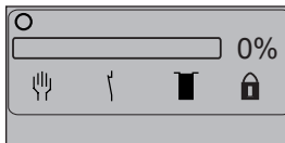
Fig. 26: Start screen with activated password protection
