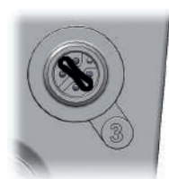
Fig. 22: Conductive rubber band in connection socket 3
