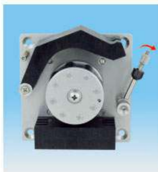
1. Turn the spanner clockwise.
