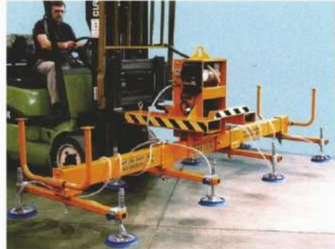
Bataryalı, forklift tipi vakumlu taşıma sistemleri Battery operated, forklift mounted vacuum lifters
